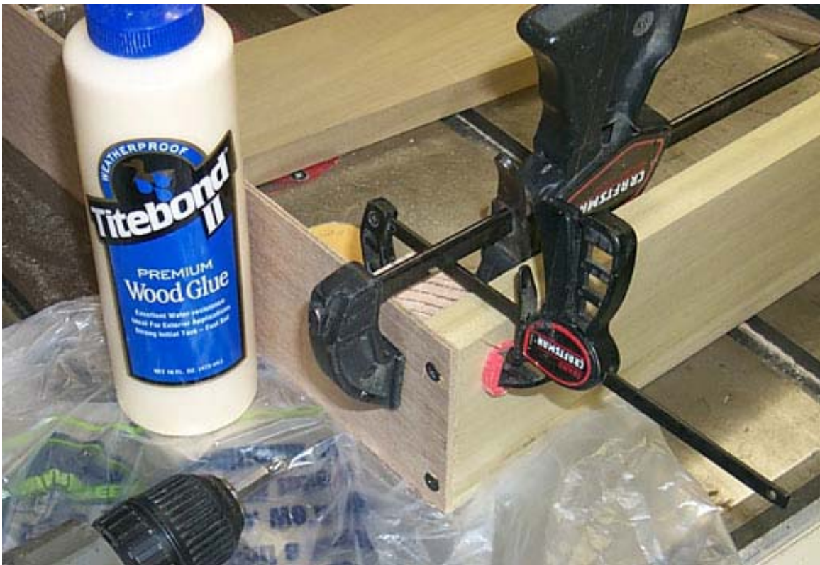
Sides overlap the ends and are joined with glue and screws. Clamps and a temporary block aid assembly.
